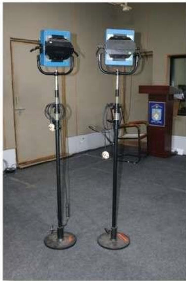
60 W LED JET LIGHT WITH 5600K WITH 95 CRI, 25 DEG BEAM ANGLE WITH DIFFUSER & SOFT BOX
